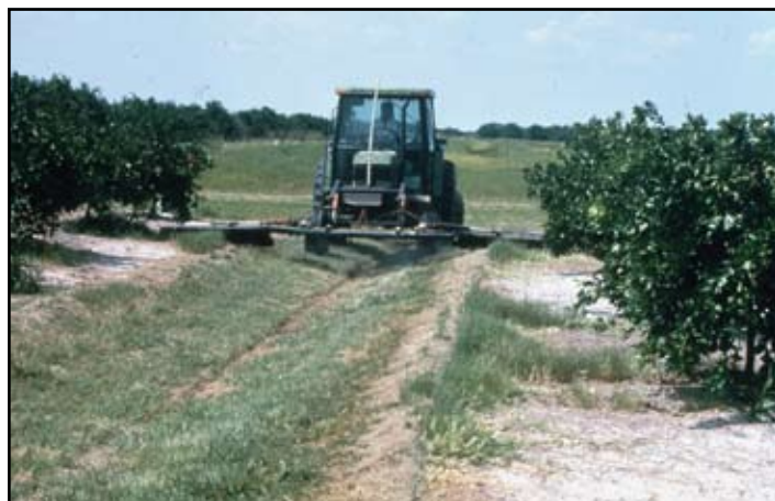
Fig. 7.4. Boom applicator used to apply suspension fertilizers. (Stephen Futch)
