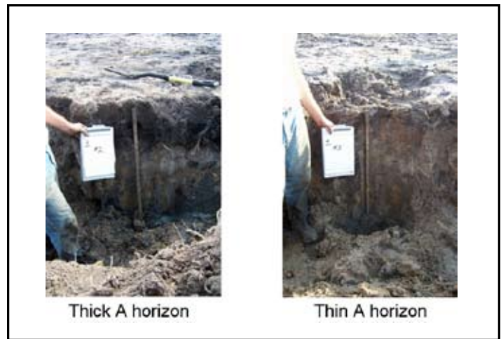
Fig. 2.8. Effect of leveling a flatwoods citrus site on topsoil (A horizon) thickness. Note the thick, dark topsoil on the left and lack of same on the right. (Mace Bauer)
