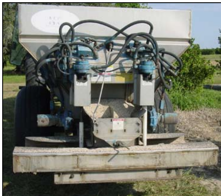
Fig. 7.1. Conventional fertilizer spreader equipped with a split chain and rear deflector plates to apply dry, solid fertilizer beneath the citrus tree canopy. (Mongi Zekri)
