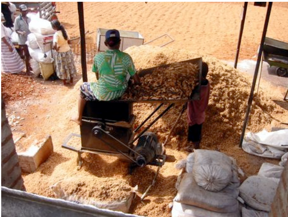
Coconut fibre or coir substrate, it's obtained, in the Sri Lanka Island, from the crushing and processing (picture above) of the external part of the coconut fruit, Coccus nucifera (picture below). It is a by-product of the extraction industry of the fibre and is composed exclusively of lignin and cellulose.
